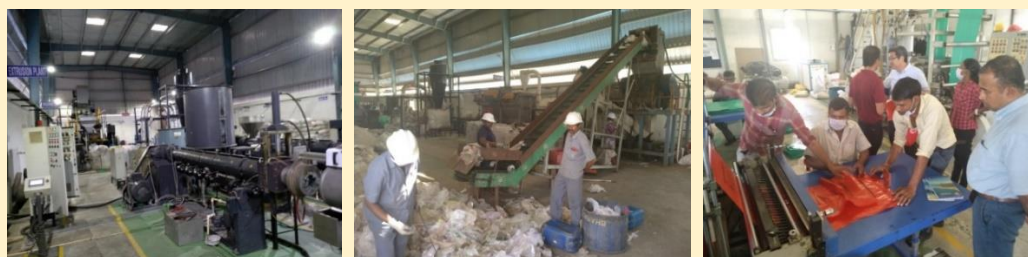
Figure 7: Washing plant (left), extrusion plant (center) and recycled plastic product manufacturing (right)
