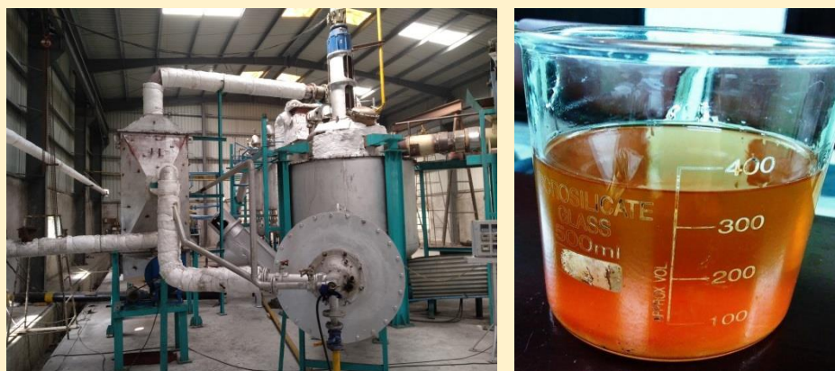
Figure 12: Pyrolysis Plant in Hyderabad (left), Distilled Furnace Oil Produced in Pyrolysis Plant (right)
