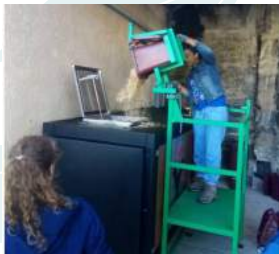
A bucket of Bokashi is poured into the electromechanical composter, la Fumainerie, Bordeaux. Source: MAMMO
